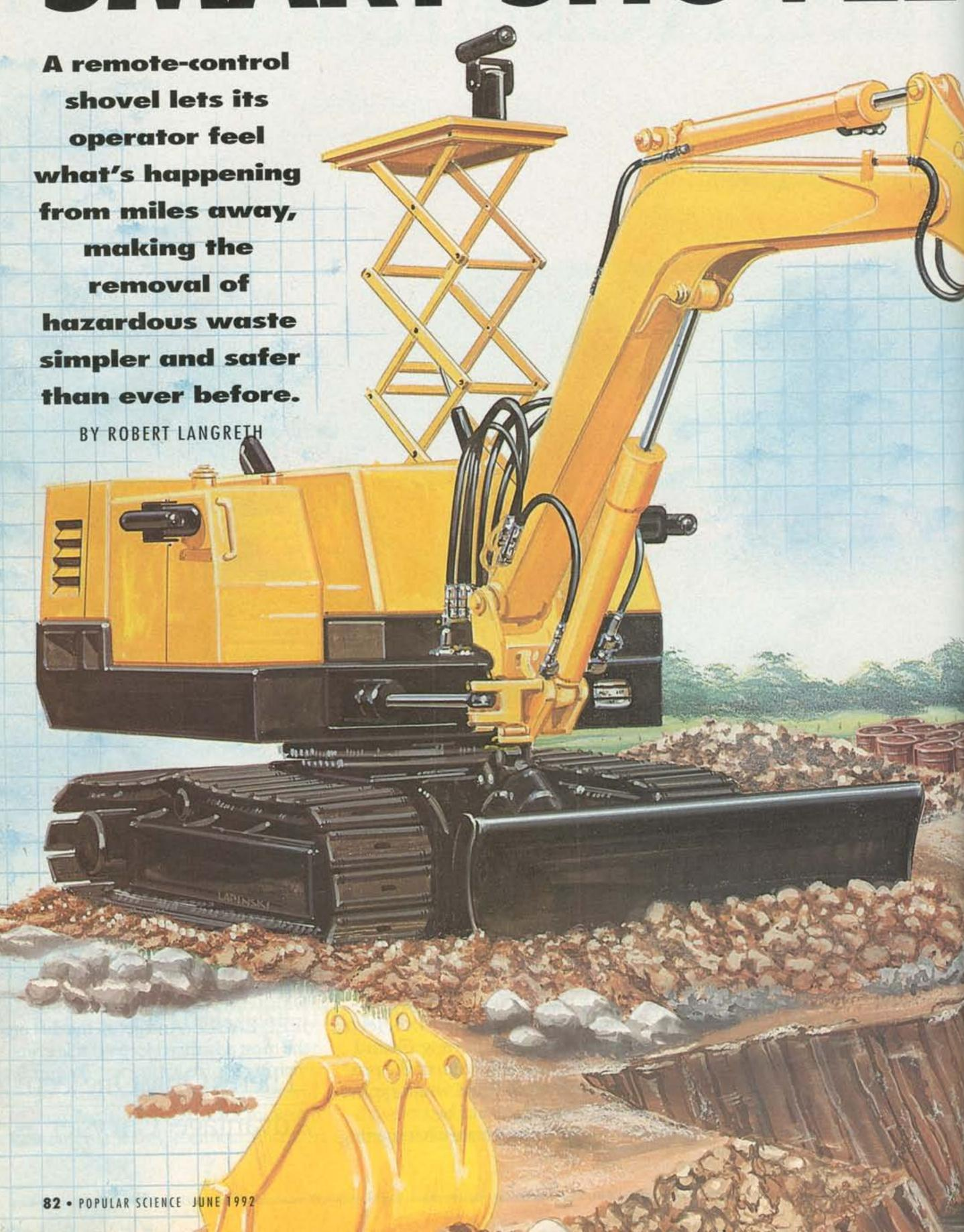
erched in the middle of a radioactive waste site, the giant yellow machine looks like an ordinary hydraulic excavator, except there is no operator, or place for an operator. The only sign that humans might be watching are three cameras mounted on a platform above the engine.
